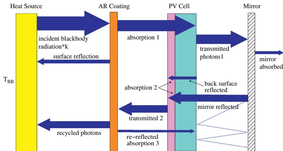
Fig. 3. Schematic diagram of the thermophotovoltaic computational model.
