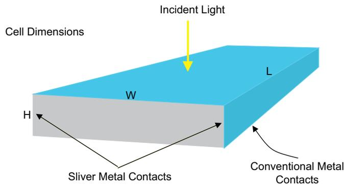
Fig. 4. Cell contact location.
